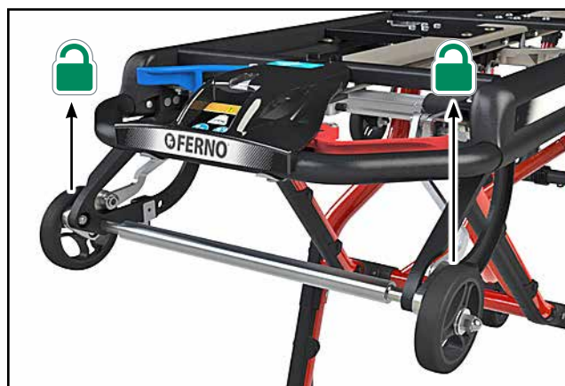
Figure 10 - Pressure On the Loading Wheels Unlocks the Loading-End Legs
